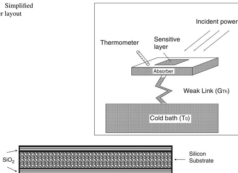
**Fig. 16.2** SiO<sub>2</sub> thermally grown by CVD on the c-Si wafer
